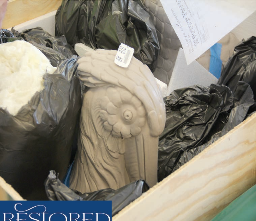
(above and below) The chimera visible between the packaging showcase the extraordinary level of detail provided by Boston Valley Terra Cotta when crafting the new chimera. From feathers to wrinkles, the detail is a byproduct of a team of artists who hand carve each detail.
